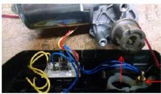
Remove motor carriage from plastic housing
