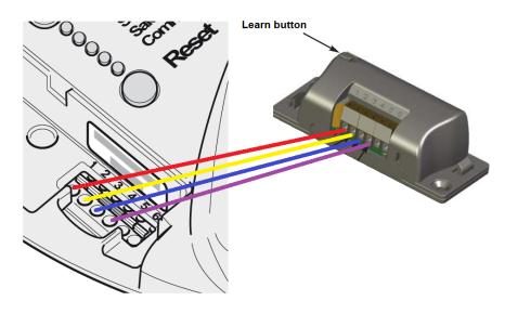
Press the Learn button on the receiver, if powered correctly, the receiver will "click" and a LED will light up inside.
